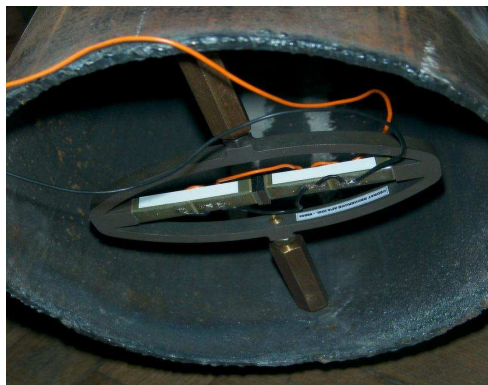
FIGURE 8. Piezo-driven actuator inside the tube specimen.
